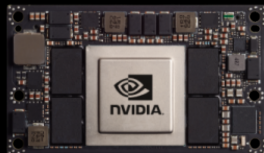
JETSON TX1 → JETSON TX2 4 GB 7 - 15W 1 - 1.3 TFLOPS (FP16) 50mm x 87mm $299
