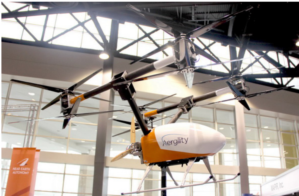
The Aergility Atlas Cargo UAV generates electric power with a bank of autogiros mounted above the vehicle.
